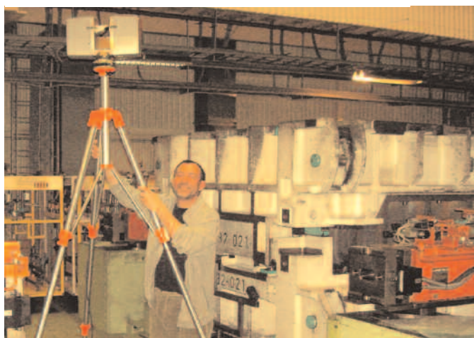
Scanner in position for overview scan
