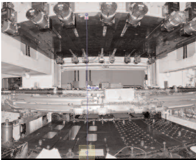
Scan data of detail inside transfer press
